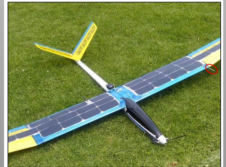
Figure 4: Layout of Solar Cells on a Glider Plane
